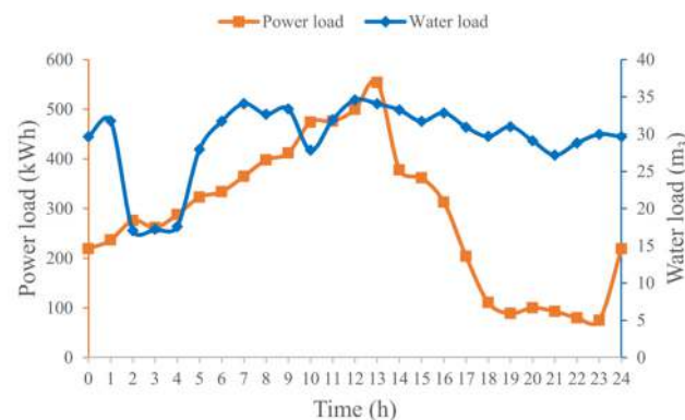
Figure 3. Hourly water load and power load for the case study [26].
